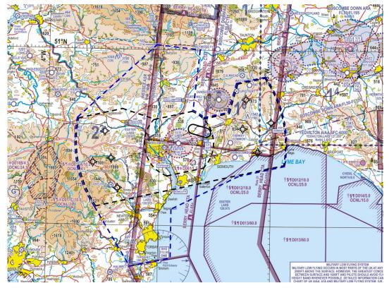
Figure 29 – 6x5 Lozenge and IAF-Protected Expanded Zone plus Upper Zone to the North and South Avoiding Dunkeswell
