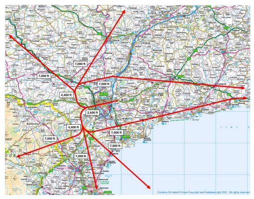
Figure 5 – Runway 26 Extended Standard Instrument Departures (OS Mapping)
