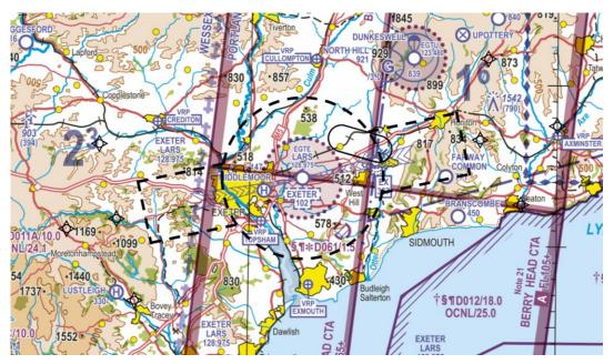
Figure 14 – 5 nm Circle with 4 nm Wide Stubs
